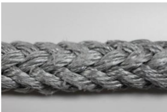
Abrasion examples – acceptable level of wear.
